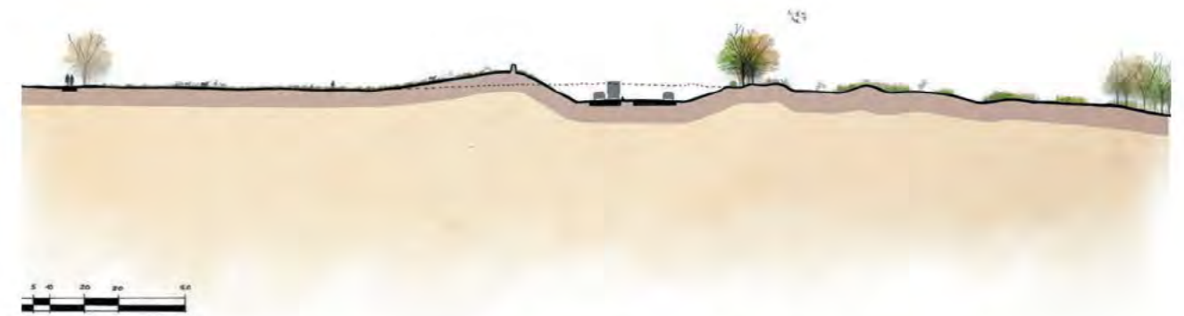
Illustrative cross section of the scheme set into the landscape, enclosed by landscape bunds
